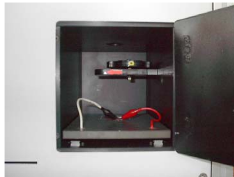
R/G/B/White Color filter without rotation stage
