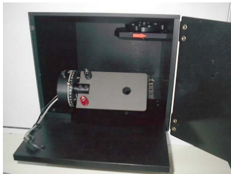
R/G/B/White Color filter with rotation stage
